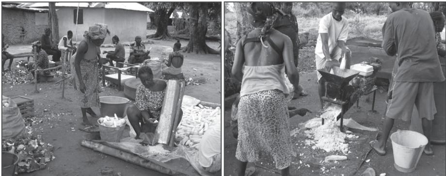
Figure 4. Using traditional hand-graters (left) and the generator-driven mechanized grater (right) in gari production, Kpetema village, XXX District, May 2008 (author's photographs).
